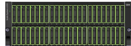
Single FCM Tier + Fully Populated (48) Drive Configuration
