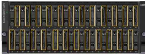
Single NVMe Tier + Half Populated (24) Drive Configuration
