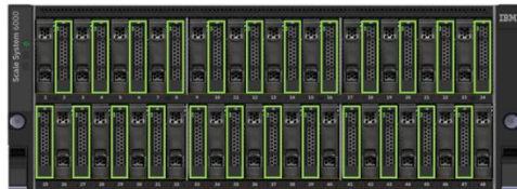
Single FCM Tier + Half Populated (24) Drive Configuration
