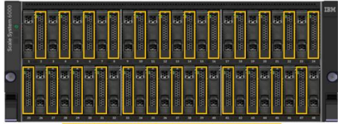
Single NVMe Tier + Half Populated (24) Drive Configuration
