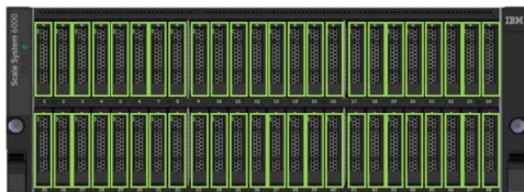
Single FCM Tier + Fully Populated (48) Drive Configuration
