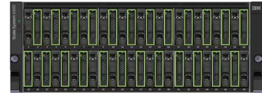
Single FCM Tier + Half Populated (24) Drive Configuration
